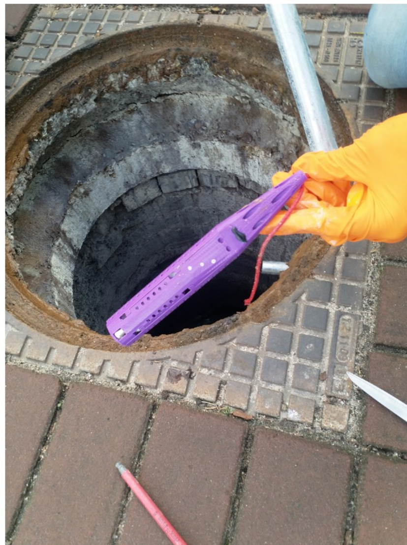
Illustration 1. A passive sampler is collected from the wastewater after 48 hours of sampling.
